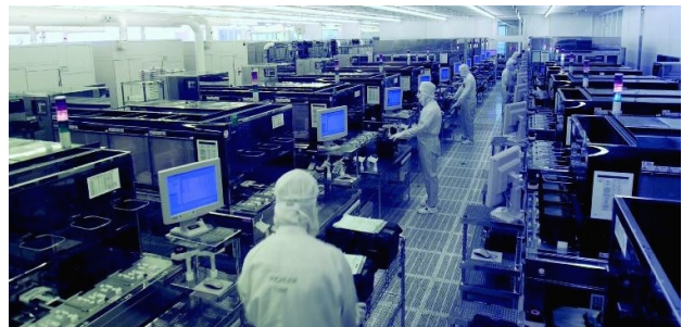
Figure 1: Clean room in a semiconductor factory. Operators are wearing suits and rubber gloves in order to reduce dust circulation.
