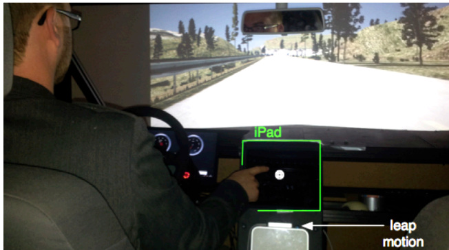
Figure 2. Physical setup of the interaction. Participants were asked to acquire the target object repeatedly during driving in a car simulator. The 3D sensor was positioned in a way that would allow to sense mid-air finger movement before participants touched a target on the screen.
